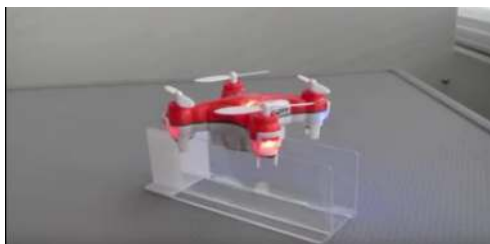
Prototype pollination drone. Photo: Eijiro Miyako
