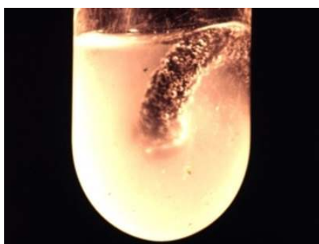
Elastomer o-ring dissolving in supercritical CO 2 Photo: Martyn Poliakoff
