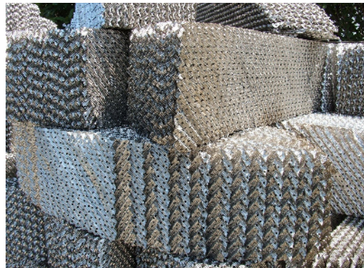
Dense structured packing for use in scrubbers. As Venus's gravity is similar to Earth's, the Ergun equation for calculating the pressure drop through a packed bed can be expected to be roughly valid. 144
