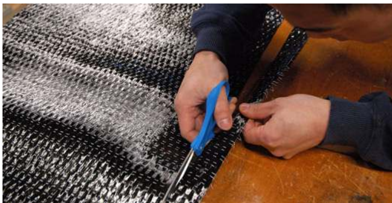
Cutting carbon fibre cloth for a layup. Photo: SkiBuilders.com
