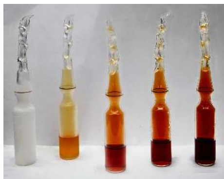
Nitrogen dioxide at different temperatures. Photo: Efram Goldberg
