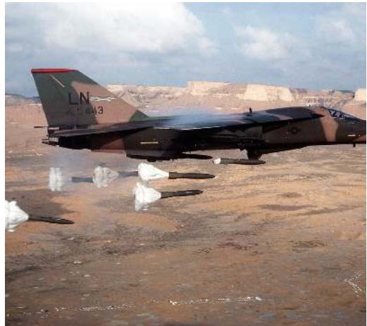
Mark 82 high-drag bombs utilize a ballute for deceleration from high speeds. Photo: USAF
