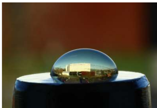
1-ethyl-3-methylimidazolium tetrafluoroborate, an ionic liquid, on polyethylene. Photo: Indrek Must
