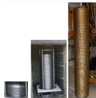
0.8m diameter bellows. Image: NASA / JPL-Caltech
